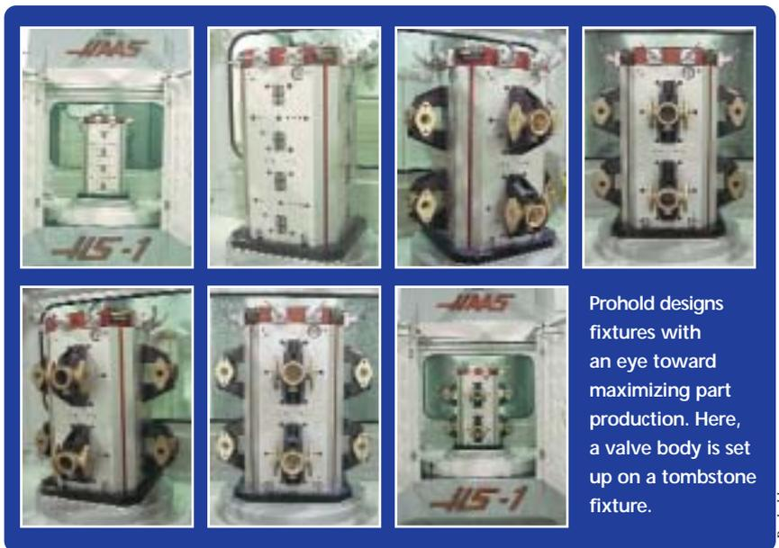
Prohold designs fixtures with an eye toward maximizing part production. Here, a valve body is set up on a tombstone fixture.
