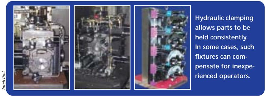
Hydraulic clamping allows parts to be held consistently. In some cases, such fixtures can compensate for inexperienced operators.
